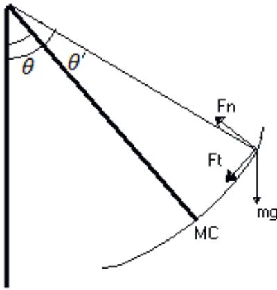
In order to study easily the behavior of the attraction, we are going to suppose that its movement is the same of a pendulum.
