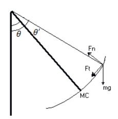
In order to study easily the behavior of the attraction, we are going to suppose that its movement is the same of a pendulum.
